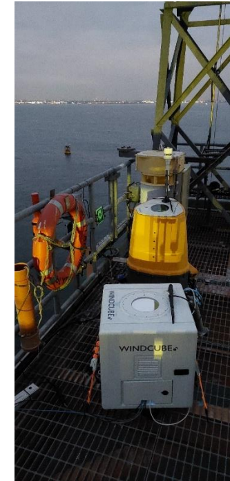
NOAH (National Offshore Anemometry Hub) met mast / test site with two fixed lidars on platform
