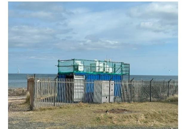
Scanning lidar in pairs as Dual-Scanning Lidar (DSL) at C-Test (Centre for the Testing of Environmental Sciences Technology), pointing at NOAA
