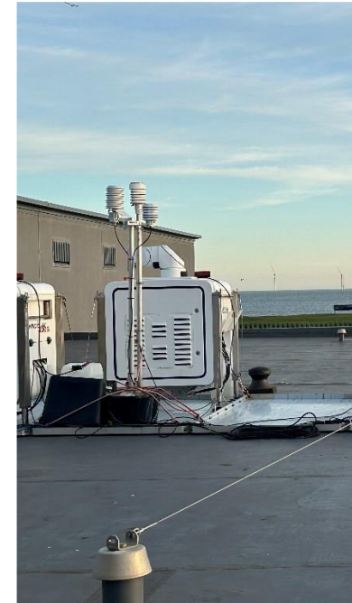
Scanning lidar in pairs as Dual-Scanning Lidar (DSL) at C-Test (Centre for the Testing of Environmental Sciences Technology), pointing at NOAA
